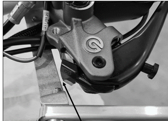
Pull clutch in all the way and ENSURE there is at least 2-3mm clearance between the mounting bracket and inner end of clutch lever
