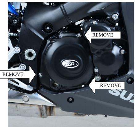
In this kit there should be: 1x Engine Case Cover (ECC0202) 3x M6 x 1.00 x 40mm CAP HEAD BOLTS
