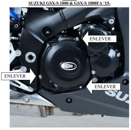
$\label{eq:linear} \begin{array}{l} \mbox{Le kit doit contenir:} \\ \mbox{1 x Protection carter moteur (ECC0202)} \\ \mbox{3x} \quad M6 \ x \ 1.00 \ x \ 40mm \ \mbox{Boulons} \end{array}$
