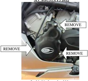
In this kit there should be: 1 x Engine Case Cover (ECC0146) 3 x M6x30mm long button head bolts 3 x M6 Washers
